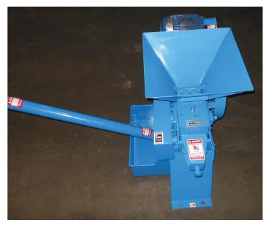
Your pencil auger can be used with the Econo mill, or we can custom-build you one to the length you need. Common sizes are 4" and/or 3" augers. Pictured above with an auger boot
